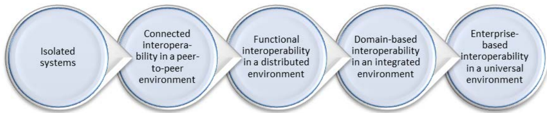
Figure 3. Stage model for the development of interoperability in an application environment
